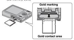
Align the gold marking with the gold contact area, then insert an SD Memory Card completely.
