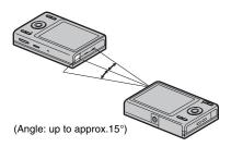
(3) Point the camera's infrared port towards the front of the camera's infrared port (→p.12). Transmission distance is about 5 to 20 cm (2 to 7.9 in.) within approx. 15°.
